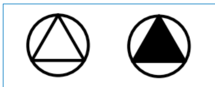
Figur 3.10 Pumpstation/tryckstegring respektive LTA-pump
