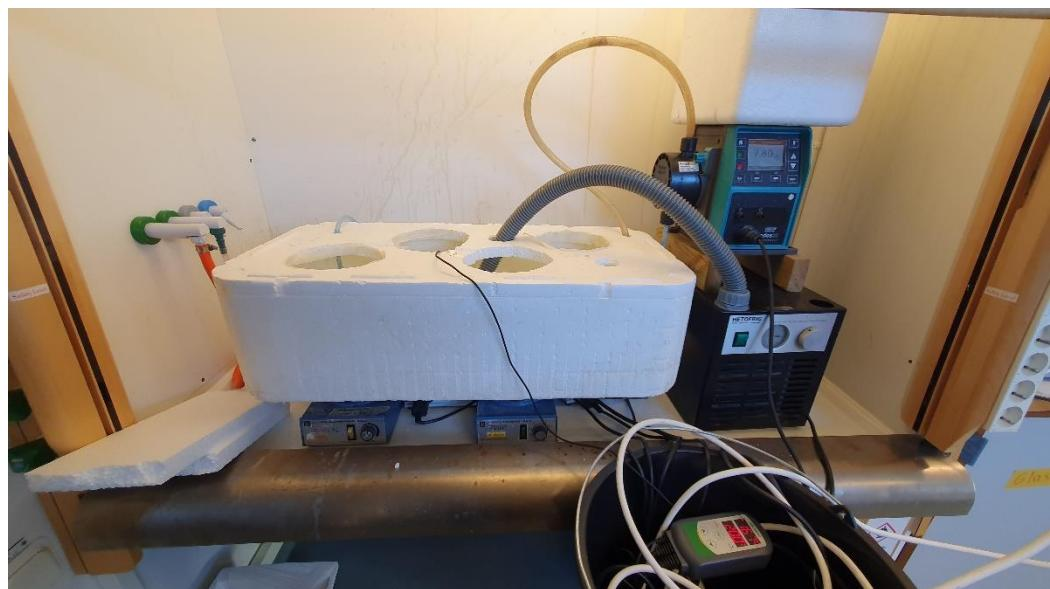
Figure 20. The water bath which has a cooling apparatus controlled by a temperature sensor.
